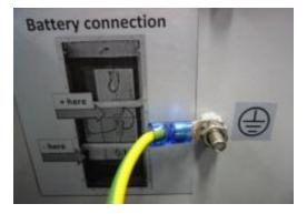
Pic. 5: Portable box LOWER part with Pic. 6: PE-Connector within portable box batteries LOWER part
