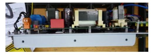
Pic. 17: Main electronic components on power board on heat sink
