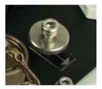
Pic. 13: Ground connector screw
